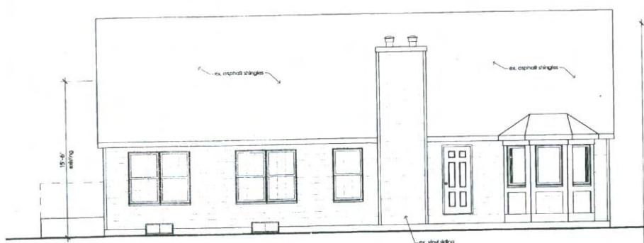
rear (west) elevation SC: 1/4" = 1'-0"
